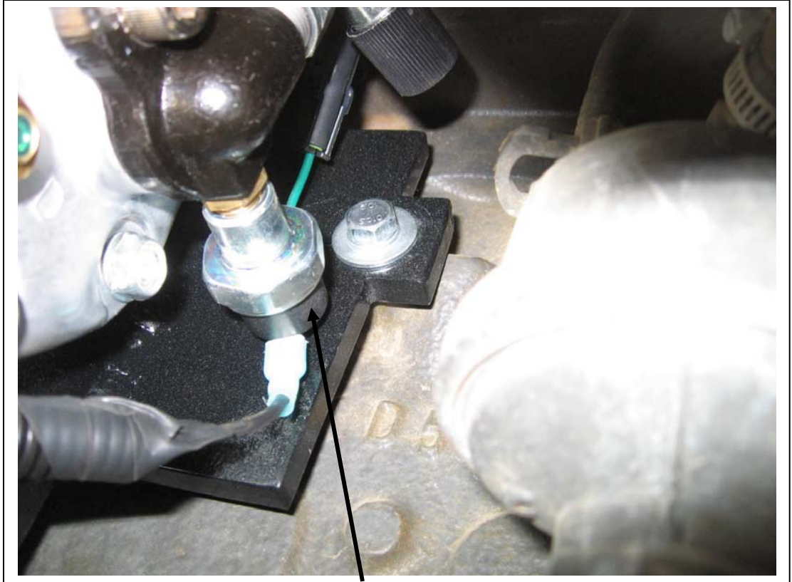
Female binary switch with wiring connected. Terminals must be bent at 90^{\circ} to connect wires.
