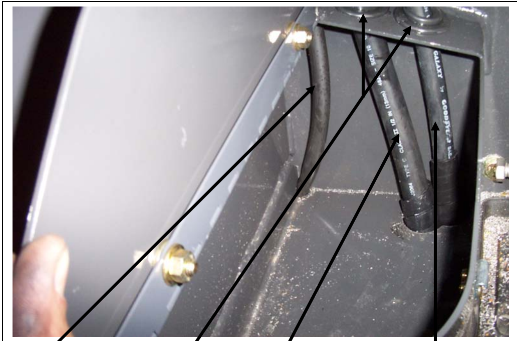
5/16" hose from the drier going under the cab to the holes drilled in the bottom of the storage box.
