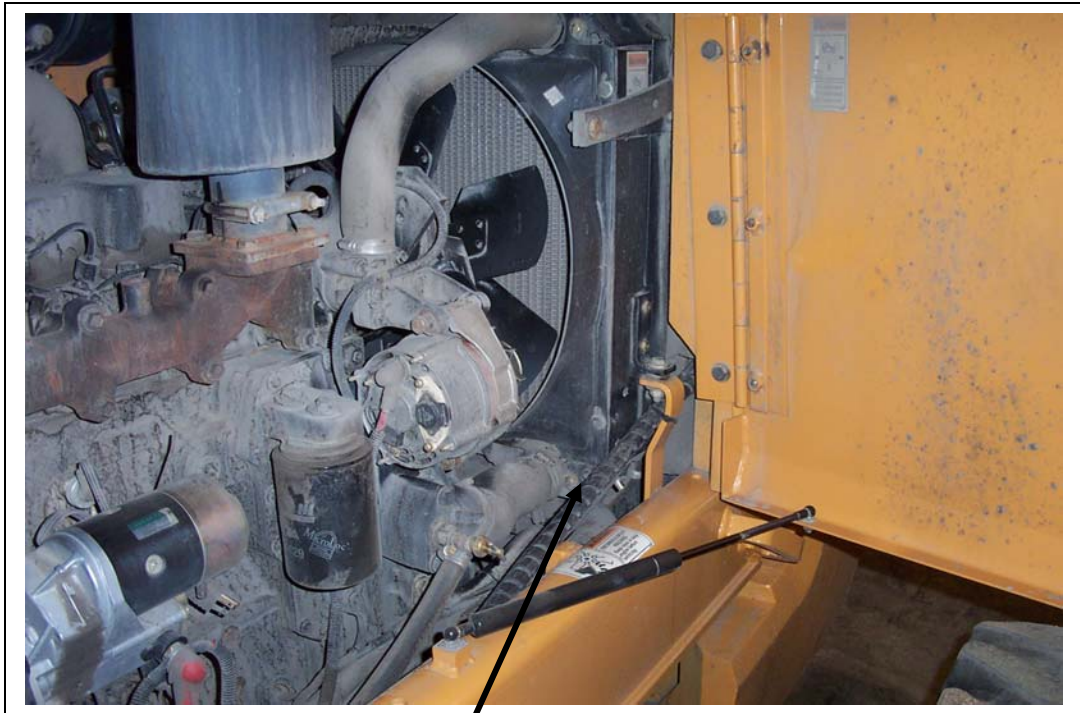
5/16" hose running forward from the condenser to the receiver drier.
