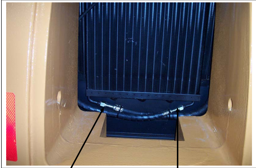
13/32" hose connected to the 13/32" condenser fitting on the left side of the coil.
