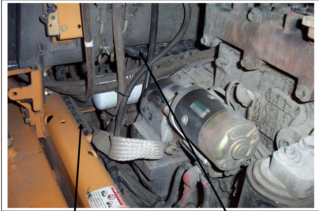
5/16" hose from the drier going under the cab to the holes drilled in the bottom of the storage box.
